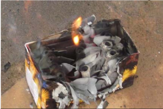
Fountain Casing continues to burn after testing.
