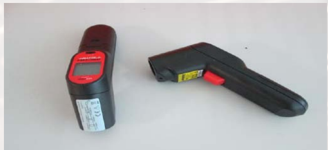
Thermal Detector used to measure internal temperature of Fountain.
