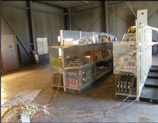
Setup of three retail shelves stocked with full Class C consumer fireworks with covered fuses, flame breaks, and restraints to limit movement of aerial devices.
