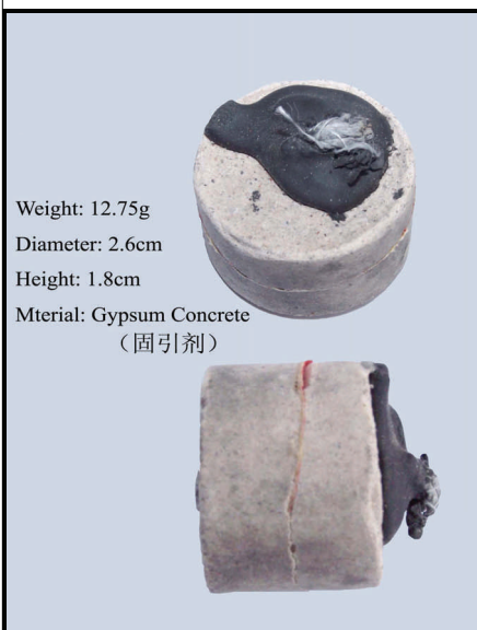
Photographs of different materials currently being used by factories in the manufacture of aerial shell inserts. Materials likely to fail the new AFSL Standard include concrete composites; clay with a binder to harden it; rigid plastic, saw dust with a glue binder, wood, or metal.
