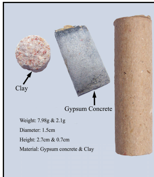
Photographs of different materials currently being used by factories in the manufacture of aerial shell inserts. Materials likely to fail the new AFSL Standard include concrete composites; clay with a binder to harden it; rigid plastic, saw dust with a glue binder, wood, or metal.
