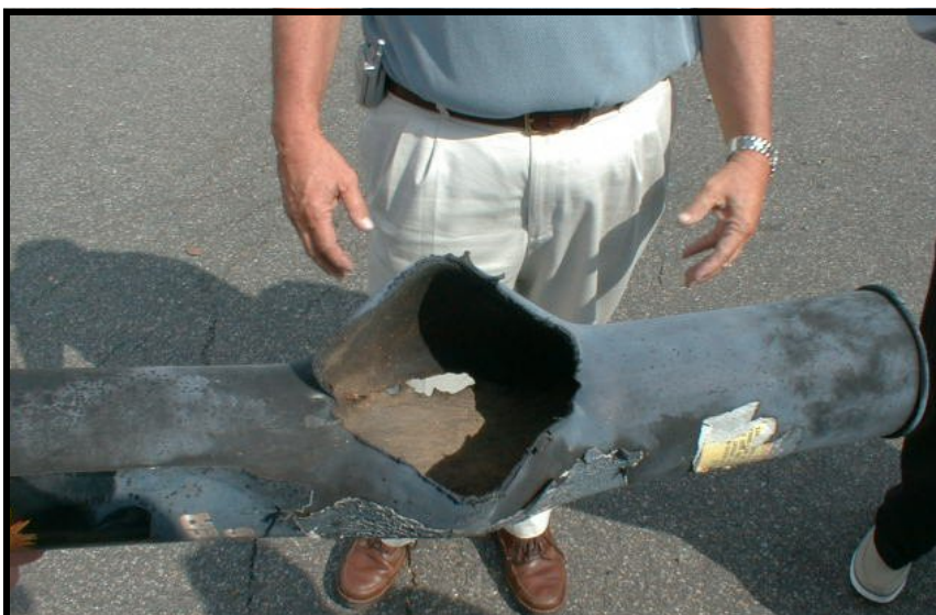
Plastic reloadable tube that experienced severe blowout and warping when shell functioned upside down inside the launcher tube.
