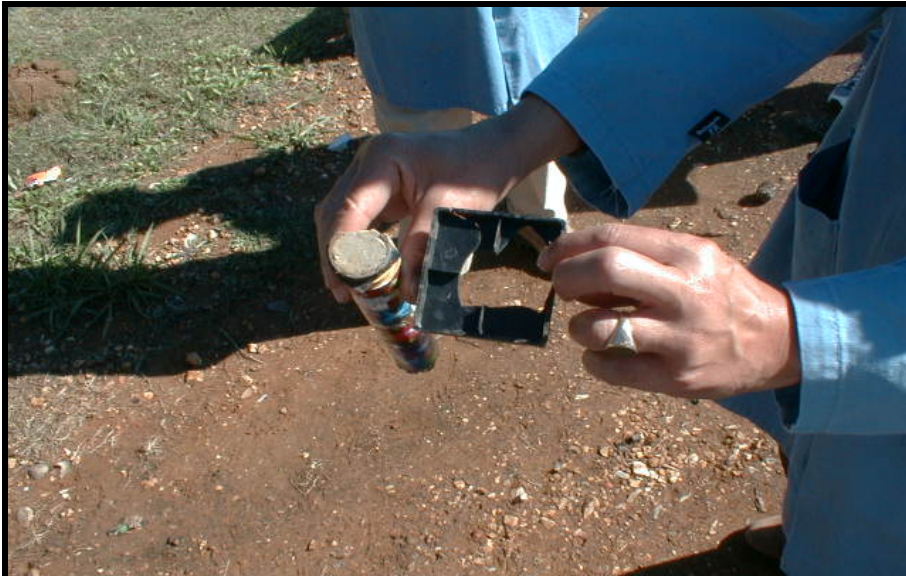
RELOADABLE SHELL TUBE THAT EXPERIENCED BASE SEPARATION AND FRAGMENTATION WHEN SHELL WAS CAUSED TO MALFUNCTION INSIDE THE LAUNCHER TUBE.
